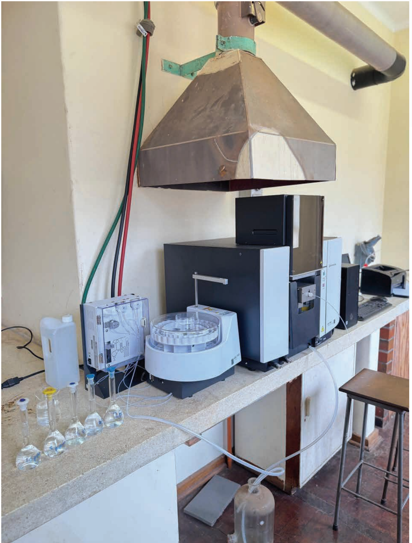
Figure 9: An atomic absorption spectrophotometer Used for mineral assaying under the Agency's mineral exploration programmes.
